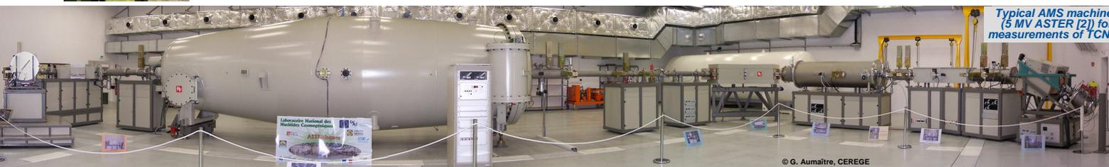
Typical AMS machine (5 MV ASTER [2]) for measurements of TCN.
