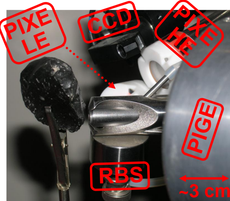
Obsidian sample in front of external proton beam (1 mm Ø) with PIXE-, PIGE- and RBS-detectors.
